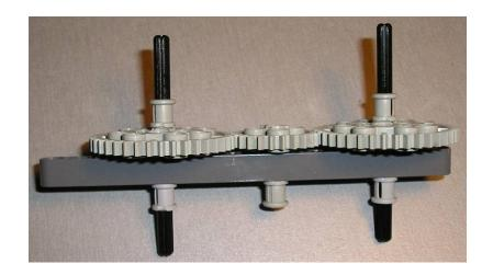
4. Take one of the assemblies built in Step 3 and attach it to the base as shown. Include an additional bushing in the location highlighted in the picture.
